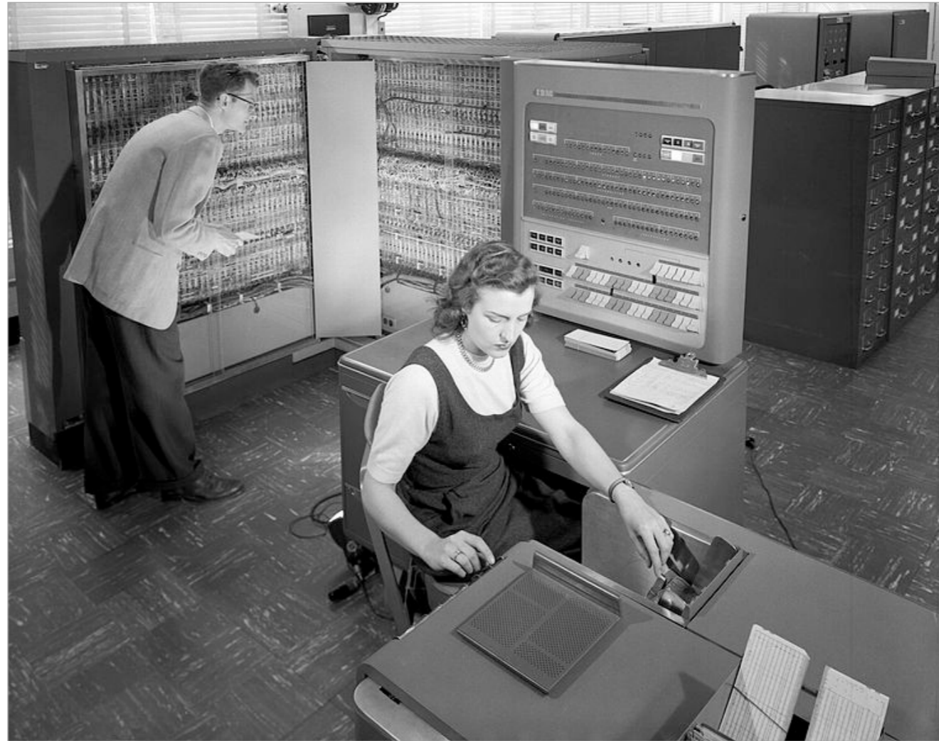
NACA researchers using an IBM 704 electronic data processing machine in 1957.
