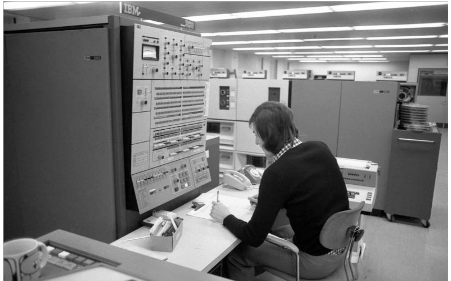
Each IBM System/360 model had the same instruction set, enabling flexibility as customers upgraded from one platform to the next. The following image is of an IBM System/360 in use at Volkswagen.
